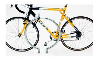
A simple circle hovering above ground, provides an artful solution for bicycle storage and security that meets Association of Pedestrian and Bicycle and Professionals (APBP) recommendations. Ring must be embedded. Ring can secure two bicycles parked parallel to the rack. The bicycles can be headed in opposite directions, or in the same direction. The rack provides two- point contact to prevent the bicycle from tipping over. A standard D-shaped bike lock can secure both a wheel and the frame.
